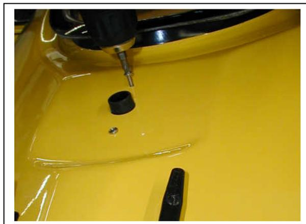
Fig. 9 – Installation of Trim Tab assembly.
