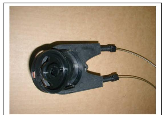
Fig. 6 – Swage slotted into spool.
