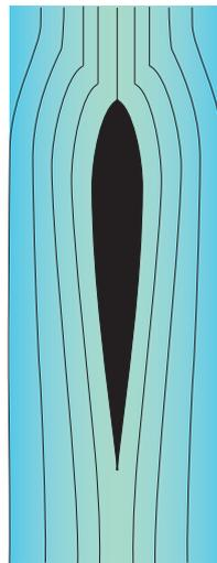
The foil shape of the blade creates more efficient water flow.
